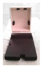
2) Install the plate to the box. The strut for cable what is mounted to the plate has to face in direction of the two holes of the box. Put the screws of the plate into the box. For easy installation lay the plate onto the cardboard box.
