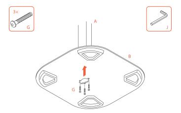
2. Attach the pole  $\circledast$  to the floor plate  $\circledast$  using the 3 x M5\*35mm bolts  $\circledast.$
