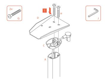
6. Attach the pole cap  $\mathbb O$  and the top plate  $\mathbb O$  to the pole  $\mathbb A$  using 2x M5\*35mm bolts  $\mathbb G.$
