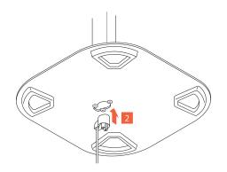
4. Push the plug with the cable guide tool B into the bottom of the floor plate B and through the pole B.
