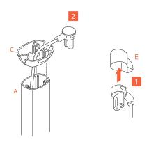
5. Remove the cable guide tool © and pull the plug through the pole cap © and put the cable in the slot on the back of the pole cap ©.
