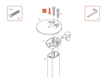
6. Attach the pole cap  ${\Bbb O}$  and the top plate  ${\Bbb O}$  to the pole  ${\Bbb O}$  using 2x M5\*35mm bolts  ${\Bbb O}$ .
