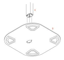
1. Put the pole a on the floor plate s.
