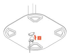
4. Push the plug with the **cable guide tool** © into the bottom of the **floor plate** © and through the **pole** ©.
