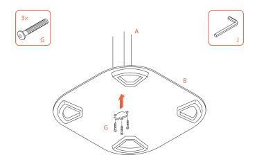
2. Attach the pole  ${\bf @}$  to the floor plate  ${\bf @}$  using the 3 x M5\*35mm bolts  ${\bf @}.$
