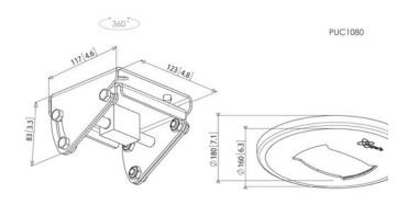
"This ceiling plate is suitable for flat and inclined ceilings (up to 60°). The display can be turned in any required position. Combine this ceiling plate with one of the poles from the Connect-it Series (PUC 2508/ 2515/ 2530), Connect-it interface bar (PFB 3405/ 3407/ 3409/ 3411) and Connect-it interface display strips (PFS 3303/ 3304/ 3305/ 3306/ 3308/ 3311) for a complete ceiling solution.
