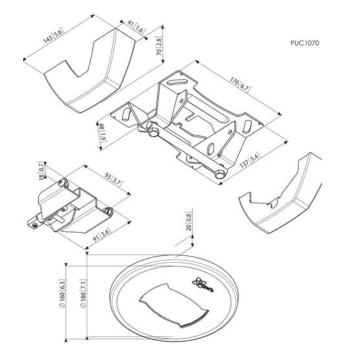
This ceiling plate is suitable for flat and inclined ceilings (up to 90°). PUC 1070 has a fixed display position to the ceiling plate and can not be turned. It is ideal for 90 degrees angled mounting in front of window or in a vide. Combine this ceiling plate with one of the poles from the Connect-it Series (PUC 2508/ 2515/ 2530), Connect-it interface bar (PFB 3405/ 3407/ 3409/ 3411) and Connect-it interface display strips (PFS 3303/ 3304/ 3305/ 3306/ 3308/ 3311) for a complete ceiling solution.
