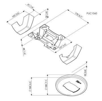
This ceiling plate is suitable for flat ceilings. Combine this ceiling plate with one of the poles from the Connect-it Series (PUC 2508/ 2515/ 2530), Connect-it interface bar (PFB 3405/ 3407/ 3409 / 3411) and Connect-it interface display strip (PFS 3303/ 3304/ 3305/ 3306/ 3308/ 3311) for a complete ceiling solution.
