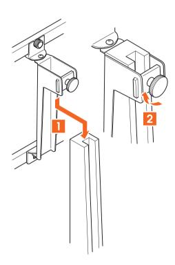
1. Slide the **steel bracket** ① over the top of the **wooden stand**  $\mathbb{R}$ . Use the knob (see illustration) to fasten the **steel bracket** ① to the top of the **wooden stand**  $\mathbb{R}$ .
