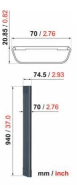
The cable covers are available in 2 widths and 3 colours. The CABLE 4 is suitable for at most 4 cables, the CABLE 8 hides at most 8 cables. Both models are supplied in white, black and anodised aluminium. Assembly is easy, a drilling template is supplied.
