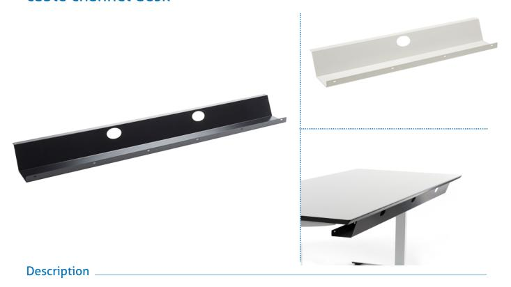
With the TecLines cable channel TKK004 / TKK005 / TKK006 / TKK007 / TKK008, confusing cable clutter at the workplace can be quickly brought under control. The desk cable guide is mounted directly on the underside of the desk top with a simple screw fastening. Inside the spacious cable tray, wires and cables can be easily bundled and securely fastened using separately available cable ties. The cable holder is available in black, white and silver and in different lengths between 40 and 147 cm.
