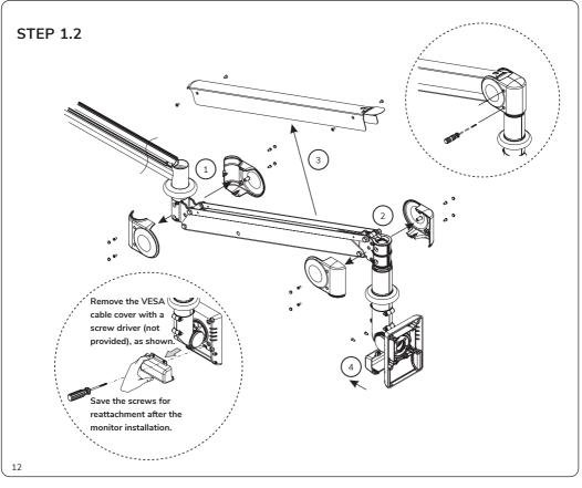
Run the cables through the arm. Assemble the cable wrapper.
