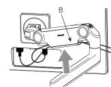
3. Slide the plastic cover (C) on the lower link upward to remove.
