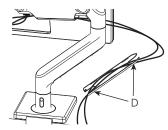
5. Lift the cover and cables up to the lower link, making sure that the cover sits flush with the surface of the arm.
