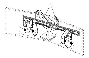
Route power and monitor cables through the flexible cable clips on the M8.1's upper link (B).
