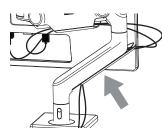
Slide the cover down the arm to lock in place, then gently pull the cables through the arm to remove excess slack
