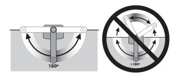
WARNING: Desk Clamp Installations: The range of motion (side-toside) for two Extensions/Arms on one pole mounted with the Desk Clamp option is limited to 180° forward (over front of desk clamp base). NOTE: Grommet Mount Installations: The range of motion (side-toside) for two Extensions/Arms on one pole mounted with the Grommet Mount option is 360°
