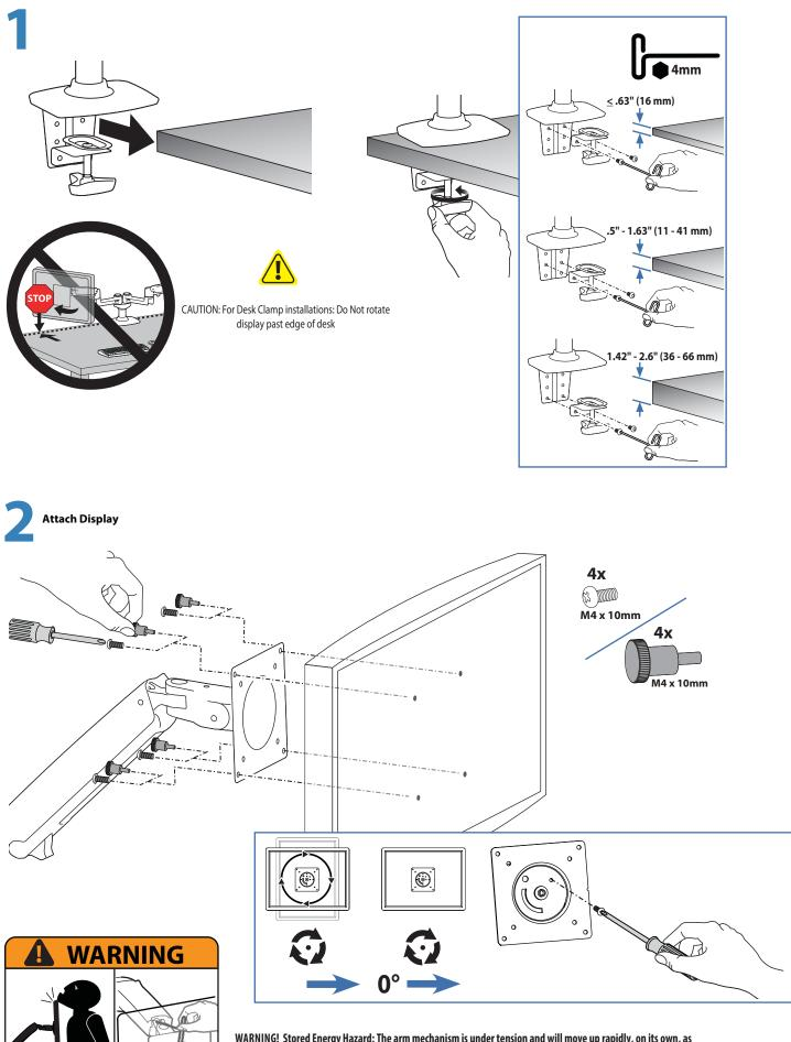
WARNING! Stored Energy Hazard: The arm mechanism is under tension and will move up rapidly, on its own, as soon as attached equipment is removed. For this reason, DO NOT remove equipment unless the arm has been moved to the highest position! Failure to follow this instruction may result in serious personal injury and/or equipment damage!
