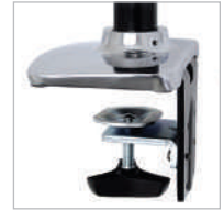
Desk Clamp attaches to surface edge .4" to 2.4" (1 to 6 cm) thick; Grommet Mount attaches through surface holes .31" to 2" (8 to 50 mm) wide and up to 3" (7,6 cm) thick
