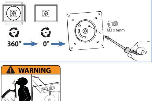
WARNING! Stored Energy Hazard: The arm mechanism is under tension and will move up rapidly, on its own, as soon as attached equipment is removed. For this reason, D0 NOT remove equipment unless the arm has been moved to the highest position! Failure to follow this instruction may result in serious personal injury and/or equipment damage!
