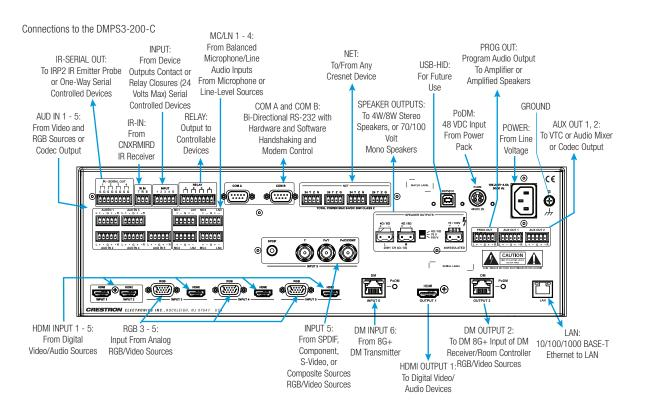
**NOTE:** Tie all source and device grounds to the ground terminal. Ensure the unit is properly grounded by connecting the chassis ground lug to an earth ground (building steel).
