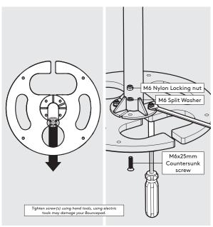
Orientate, locate and secure the Floorstanding Pole to the Floorstanding Base as shown. Ensure that all fixings are installed correctly.
