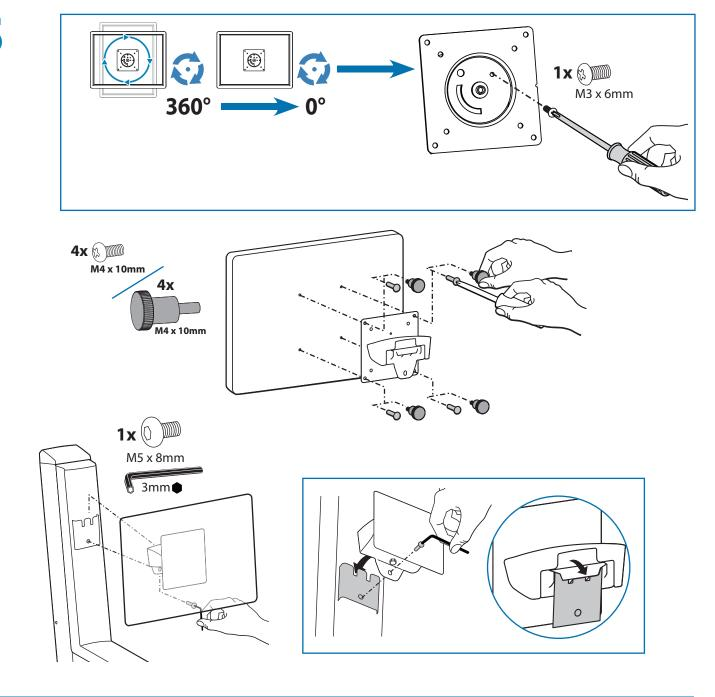
6 NOTE: Leave enough slack in cable to allow full range of motion.
