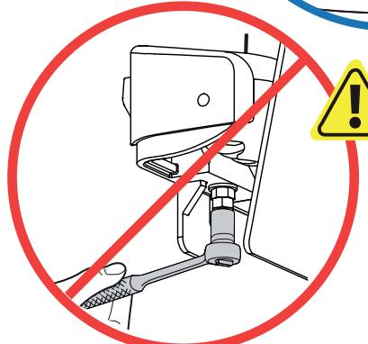
**CAUTION!** The bottom nut will turn during adjustment of the top nut; DO NOT apply any tool to the bottom nut. Serious damage to the Pivot may occur if these instructions are not followed.
